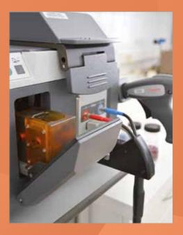
ence.for Fibre optic probes enable the analysis of materials without the opening of the primary packaging, and the microscope enables the characterization and identification of small particles, and chemical mapping characterization of surface areas and subsurfaces of various samples and dosage forms.
