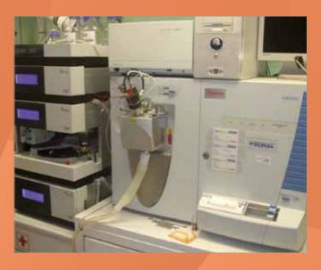
ary phase is unpolar, while the mobile phase is polar. The mobile phase is passed to the MS through an interface unit, of which ensures the ionization and desolvation too.
