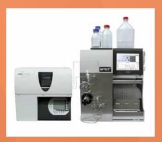
sorption on the column, the stationary phase can be evaporated allowing a 100% sample recovery, no silica waste is needed to recycle, and the solvent demand is quite low. The large number of available biphasic solvent systems ensure great optimizability, making the technique applicable on a wide scale. The instrument monitors the UV absorbance at two wavelengths, and has a built-in fraction collector programmable to collect individual chromatographic peaks separately.
