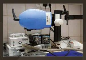
nous with these changes, cerebral blood flow maps are created based on laser speckle contrast analysis. The illumination and camera exposures are synchronized by a dedicated program created in LabView environment specifically for this purpose.
