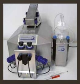
ment of the mitochondrial electron transport chain is performed by using substrate-uncoupler-inhibitor measurement protocols, which allows real time follow-up of respiratory functions. The fluorescence module can evaluate the total free radical production ( $H_2O_2$ ), mitochondrial membrane potential and calcium levels during the respirometric measurements, in the same samples.
