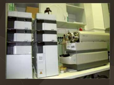
fications and quantitation while keeping cost efficiency. The mass spectrometer is very efficient in wide concentration range (5-6 orders of magnitude) due to its high sensitivity and has a good selectivity in targeted, non-targeted or unknown component analysis.
