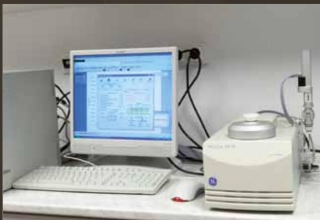
temperature, the feedback power of the reference cell can be altered. By measuring this power throughout the titration, the thermodynamical parameters can be calculated. The MicroCal VP-ITC apparatus in our lab is used to study protein-ligand interactions.
