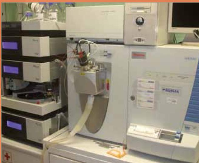
ary phase is unpolar, while the mobile phase is polar. The mobile phase is passed to the MS through an interface unit, of which ensures the ionization and desolvation too.
